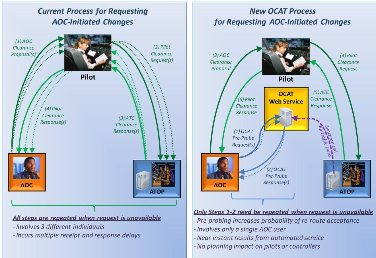
Figure 1 AOC Re-routing before and after OCAT
