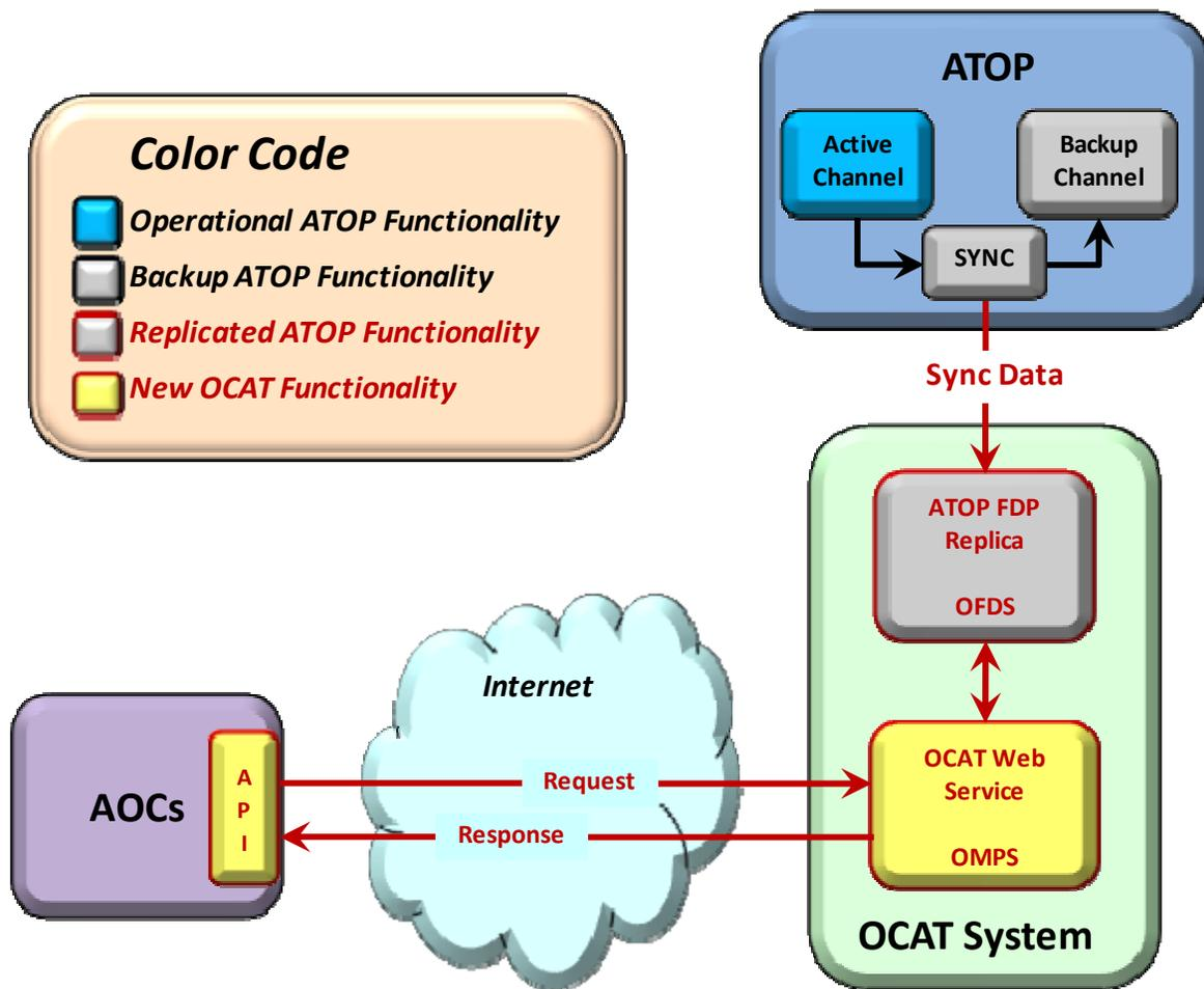
**Figure 2 High-level Representation of the OCAT Concept**
